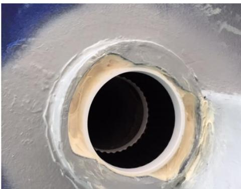
To prevent water entering the area between the bearing ball and outer housing, one can fill this up with a stiff grease. A good grease for this is Lanacote. Any synthetic grease will do the job, as long as it is as sticky and hard as butter. **Please make absolutely sure no grease gets on, or between the rollers!**
