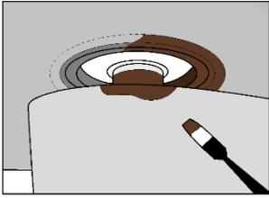
Due to corrosion on the surface, the volume of the outer housing increases and pushes the bearing ball harder on the rudder shaft creating friction and making the steering stiffer and stiffer. In most cases this is caused by using metal consisting anti-fouling too close to the bearing housing. It's very important to use nonmetallic anti-fouling (like used on sail
