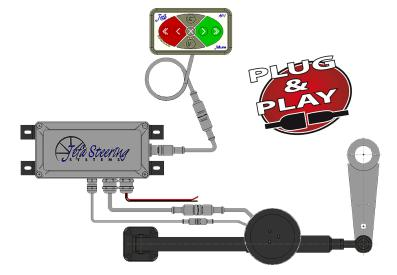
The above layout shows the super easy "plug & play" installation of the autopilot drive system. Only the plus and minus have to be connected and the drive unit, servo box and control panel are all plugged in. There is no need for a separate fluxgate compass and separate rudder feedback unit like other systems use.
