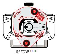
Stop ring Our stop ring fit the mounting screws under the pedestal. It can be adjusted up to 25°.
