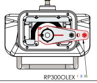
Output arm Extended output lever is used for attaching drive unit or special rudder geometry.
