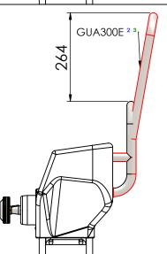
**Guardrails** For Jefas 300 pedestal, the costumer has different opportunities to choose a fitting guardrail. The top mounfed GUA300T takes less space than the standard guardrail. The extended GUA300E fits the 400 pedestal too, and has the possibility to install an instrument pod, or radar pod if needed.
